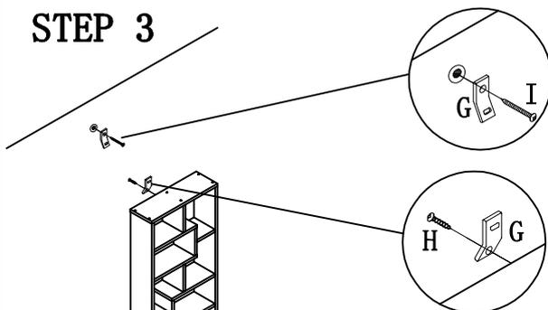
1. Insert drywall screw into metal bracket and into drywall anchor.
