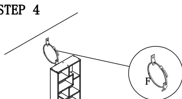
1. Insert strap thru bracket attached to wall, then thru bracket on item, and into head of strap.
