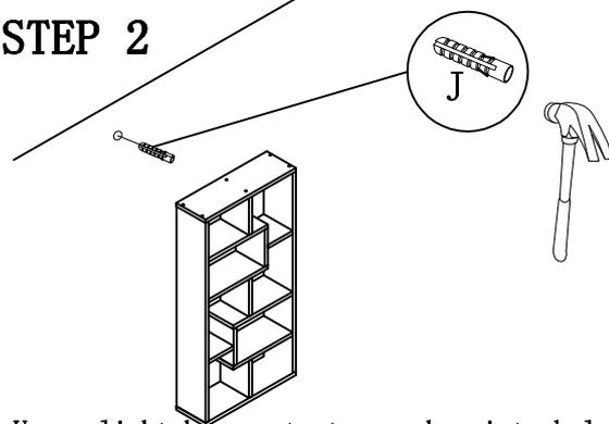
1. Use a light hammer to tap anchor into hole.
